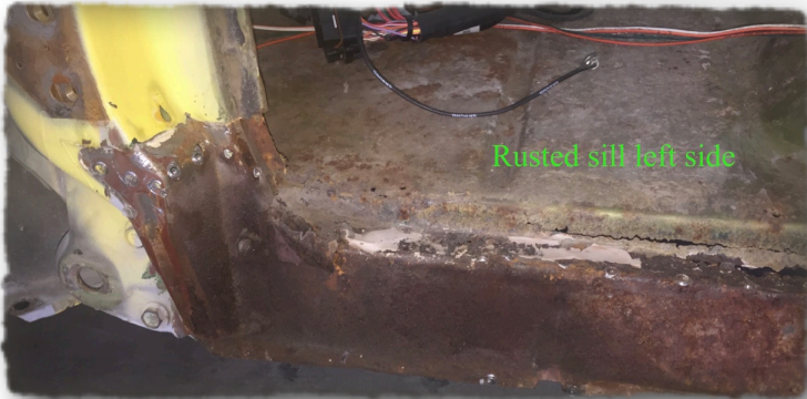
Rusted sill and floor right side
